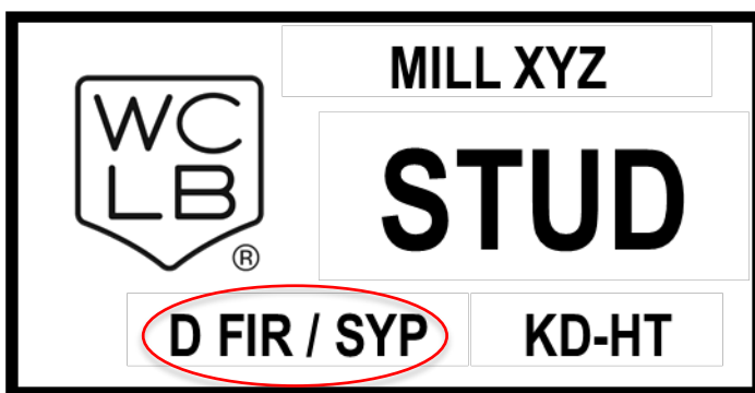
Figure 2. Example of grade stamp with two species, Douglas fir (D Fir) and Southern pine (SYP).
