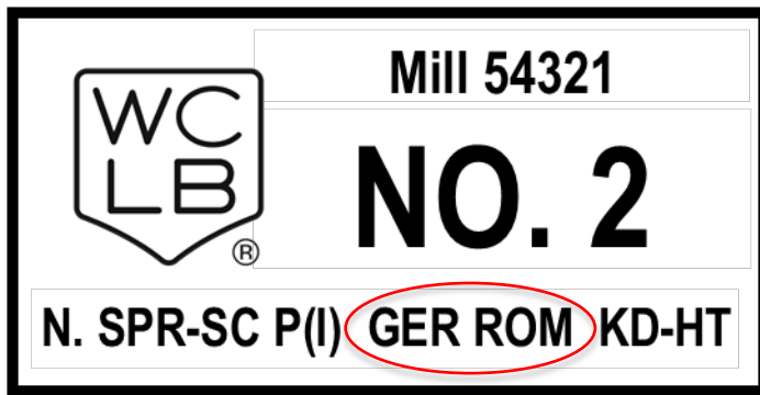
Figure 3. Example of grade stamp with two countries of origin, Germany (GER) and Romania (ROM). The (I) indicates the species are imported from outside North America.
