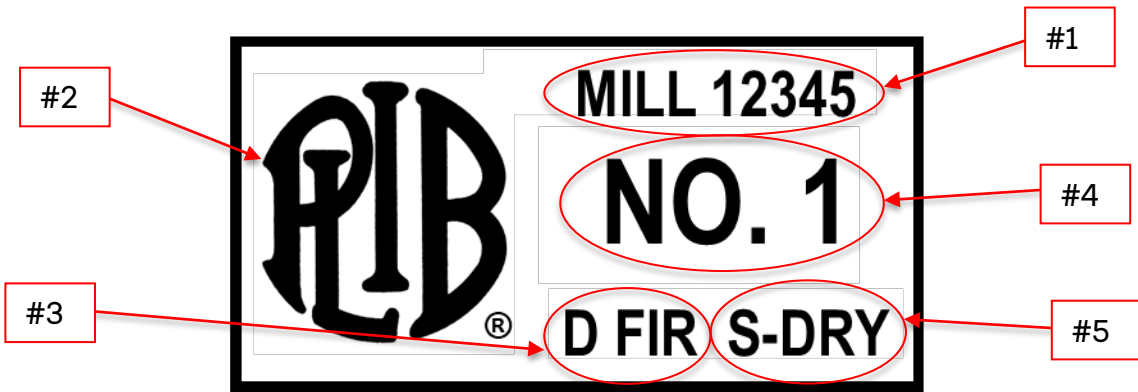
Figure 1. An example of a typical PLIB grade stamp with the five required elements.
