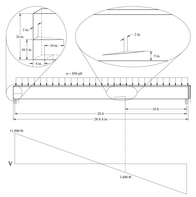
Figure 4. Example beam with load and shear diagrams.
