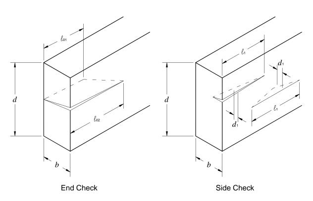
Figure 2. Determination of effective check size.
