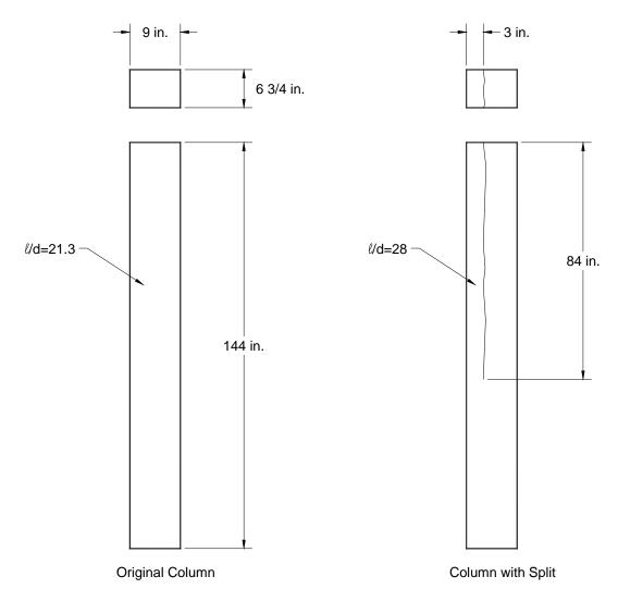
Figure 1. Effect of split on column slenderness ratio.
